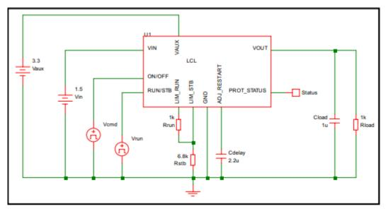
Case 2:Vin voltage is equal to 3.3V. Internal circuits are also powered from Vin.lth\_stb is set to 0.2A.lth\_run is set to 1.2A.Delay is set to 85ms.ON/OFF state and RUN/STB mode are selected by dedicated commands.
